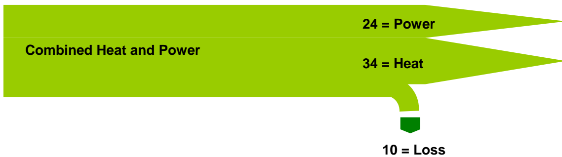
Figure 5: Energy flow diagram comparing separate heat and power plants versus 1 combined heat and power plant to accomplish both. It is evident that using combined heat and power saves 30% of the energy regardless of the energy source. 1
